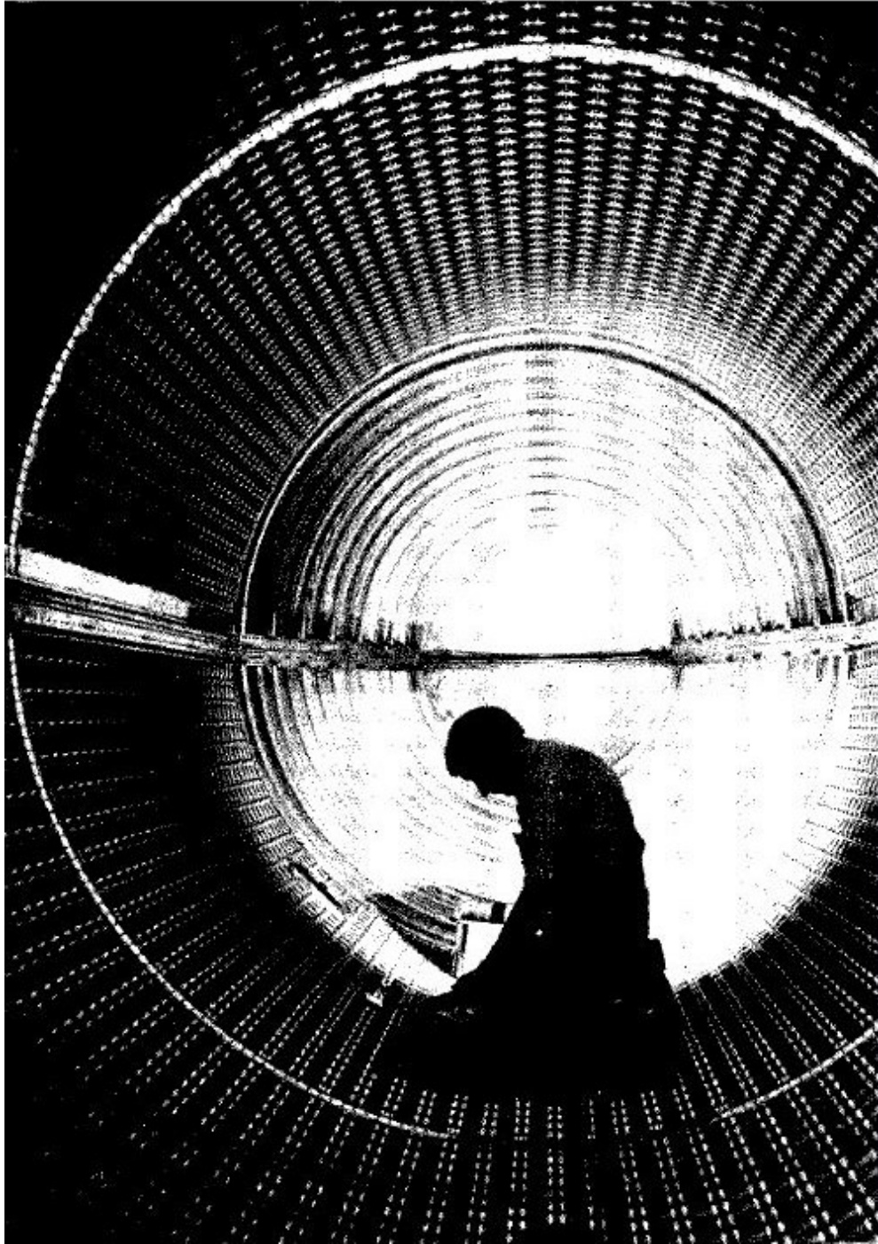
Plate II.4. The kneeling figure silhouetted by what seems to be a sparkling halo actually is a mechanic working inside the spacecraft fairing of a McDonnell Douglas Delta rocket. His portable lamp glints on thousands of facets of a triangular “isogrid” pattern milled into the shiny aluminum skin of a fairing to reduce weight while retaining maximum strength. The fairing, 8 feet in diameter and 26 feet long, protects the Delta’s payload as it is launched into orbit and from aerodynamic forces and heat during flight through the atmosphere. Courtesy of the McDonnell Douglas Astronautics Company, California.
