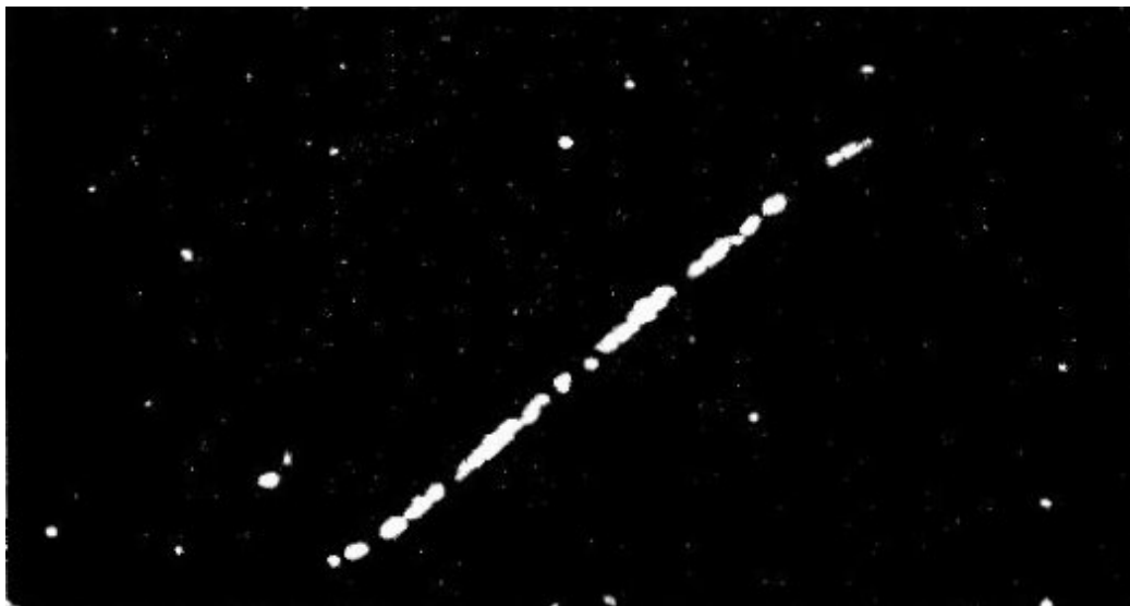
Plate III.10. Fission of a uranium atom. The white streak in the middle of this photographic plate represents the tracks of two atoms flying apart from the central point where the uranium atom split in two. The plate was soaked in a uranium compound and bombarded with neutrons, which produced the fission caught in this picture. The other white dots are randomly developed silver grains. The picture was made in the Eastman Kodak Research Laboratories. By permission of United Press International.
