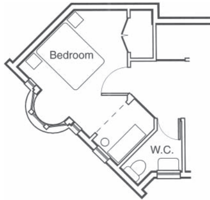
Figure 8.3 Bedroom with alcove for child's cot or study space. Vaughan Way, East London, Labo Housing Association (Homeless Minority Ethnic Families: Bengali, Somali, African-Caribbean, Chinese, Vietnamese). Architect: Matrix Feminist Architectural Co-operative. Source: Penoyre & Prasad et al. (1993), p. 37. Reproduced by permission of the Home Housing Trust.
