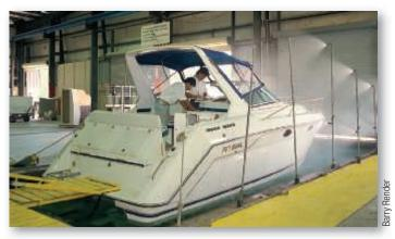
At the final stage, smaller boats, such as this one, are placed in this test tank, where a rain machine ensures watertight fits.
