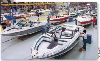
Once a hull has been pulled from the mold, it travels down a monorail assembly path. JIT inventory delivers engines, wiring, seats, flooring, and interiors when needed.
