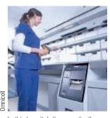
In this hospital, these vertically rotating storage carousels provide rapid access to hundreds of critical items and at the same time save floor space. This Omnicell inventory management carousel is also secure and has the added advantage of printing bar code labels.
