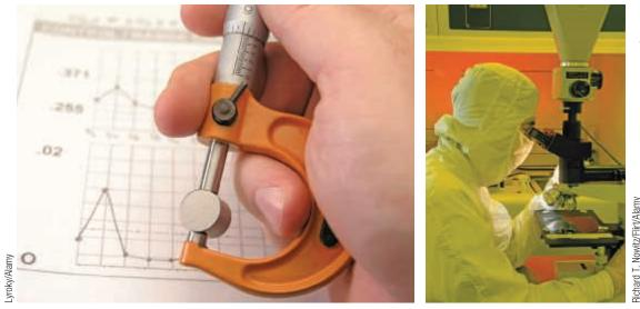
Raw data for Statistical Process Control is collected in a wide variety of ways. Here physical measures using a micrometer (on the left) and a microscope (on the right) are being made.
