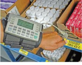
Pharmaceutical distributor McKesson Corp., which is one of Arnold Palmer Hospital's main suppliers of surgical materials, makes heavy use of bar-code readers to automate inventory control. The device on the warehouse worker's arm combines a scanner, a computer, and a two-way radio to check orders. With rapid and accurate data, items are easily verified, improving inventory and shipment accuracy.
