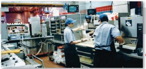
The redesigned kitchen of a McDonald's in Manhattan. The more efficient layout requires less labor, reduces waste, and provides faster service. A graphic of this "assembly line" is shown in Figure 9.11.
