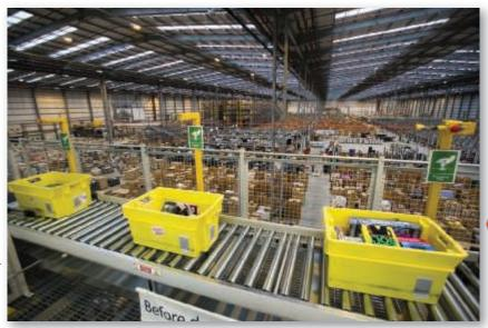
**4. Your items are put into crates on moving belts.** Each item goes into a large yellow crate that contains many customers' orders. When full, the crates ride a series of conveyor belts that wind more than 10 miles through the plant at a constant speed of 2.9 feet per second. The bar code on each item is scanned 15 times, by machines and by many of the 600 workers. The goal is to reduce errors to zero—returns are very expensive.
