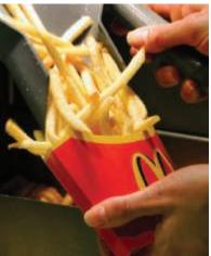
Good methods analysis and the proper tools can result in poka-yokes that improve both quality and speed. Here, two poka-yokes are demonstrated. First, the aluminum scoop automatically positions the french fries vertically, and second, the properly sized container ensures that the portion served is correct. McDonald's thrives by bringing rigor and consistency to the restaurant business.
