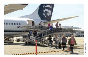
Another current Lean project is passenger unloading and loading. Lean instructor Allison Fletcher calls this "the most unique project I have worked on." One exciting aspect of deplaning is Alaska's solar-powered "switchback" staircase for unloading passengers through the rear door (see photo). Alaska is saving two minutes, or nearly 17%, off previous unloading time with this new process. Alaska Airlines' Lean culture has made it a leader in the industry.
