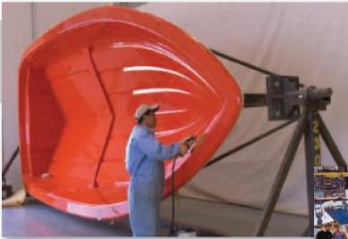
Here the finishing touches are being put on a mold used for forming the hull.
