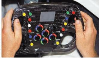
Drivers of race cars have no time to grasp for controls or to look for small hidden gauges. Controls and instrumentation for modern race cars have migrated to the steering wheel itself—the critical interface between man and machine.
