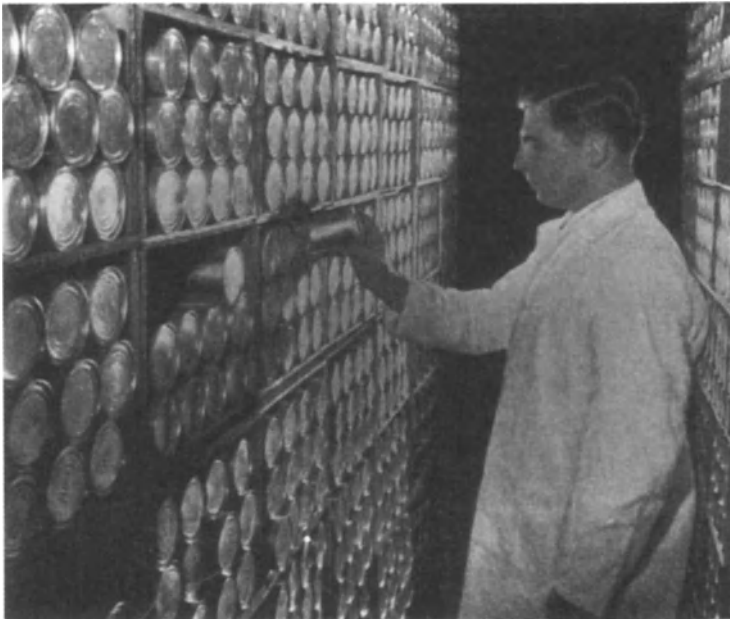
Figure 8.7. Cans being examined for bulging as evidence of spoilage. Courtesy of American Can Co.
