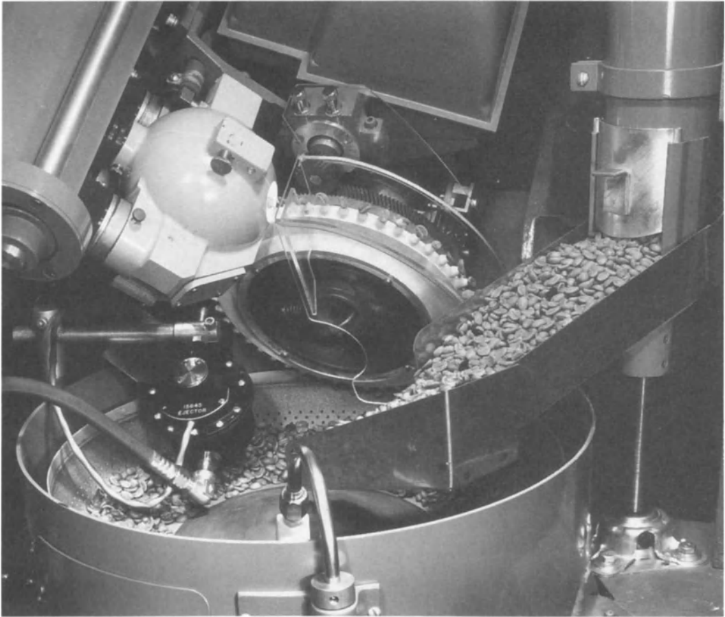
Figure 19.5. Electronic sorting of coffee beans. Other products such as peanuts can be similarly separated. Courtesy of Elexso Corp.
