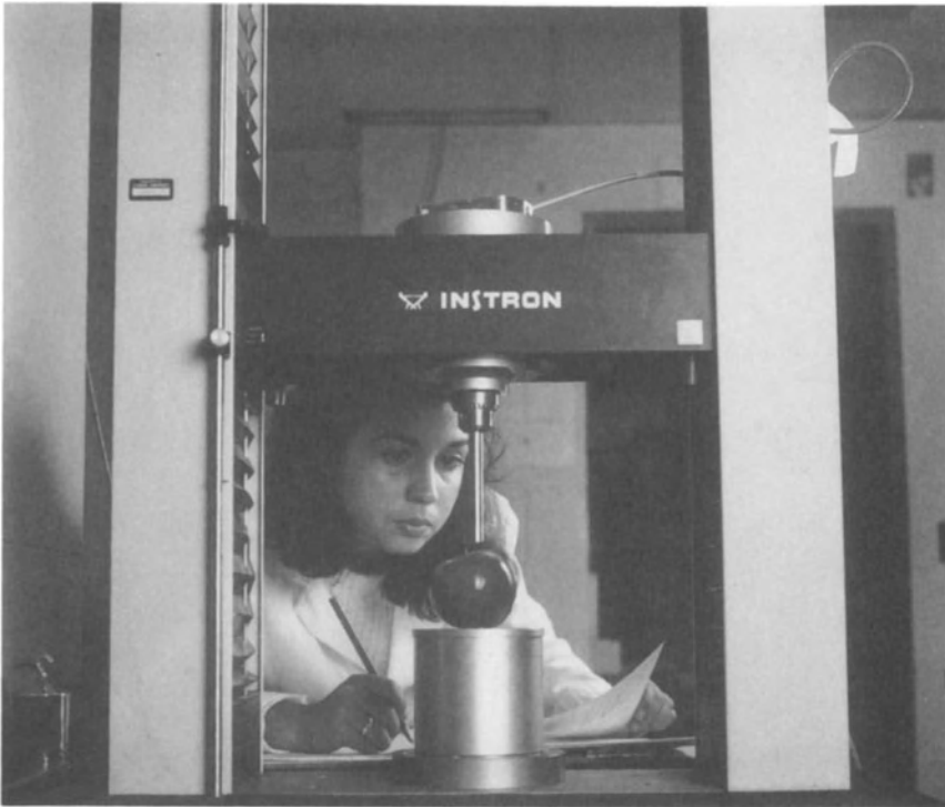
Figure 6.1. Instron Universal Testing Machine being used to test the mechanical/physical properties of an apple. Courtesy of Cornell University Photo Services.
