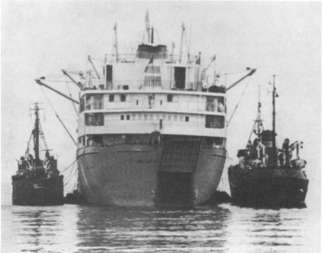
Figure 15.1. Factory ship receiving fish from trawlers for processing at sea. Courtesy of S. J. Holt.
