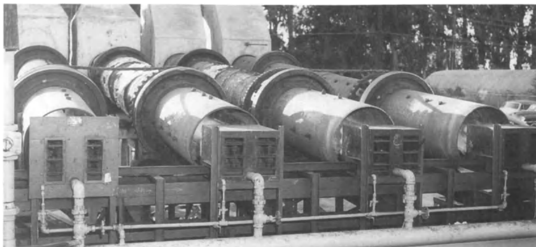
Figure 18.4. Rotary tube flame peelers for onions and peppers. Courtesy of Gentry International, Inc.
