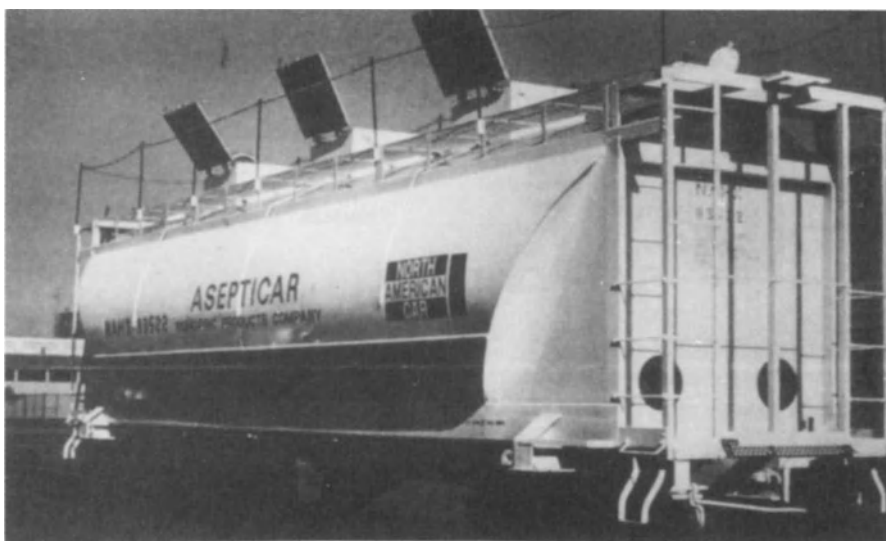
Figure 10.24. Aseptic rail car for tomato paste and other concentrates. Courtesy of Fran Rica Mfg., Inc.
