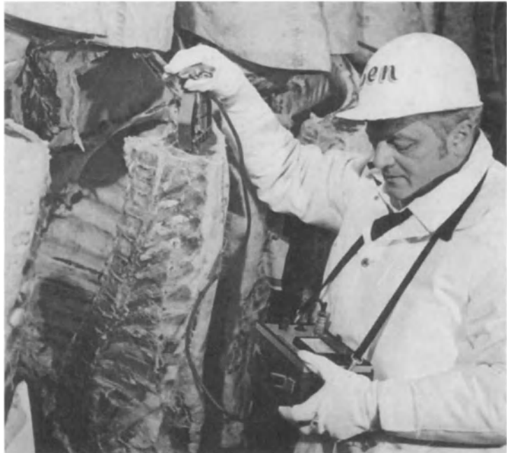
Figure 6.10. Evaluating the tenderness of beef with the Armour meat tenderometer. Source: Anon. Food Technology 27:1. 1973.
