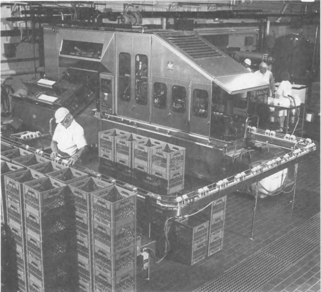
Figure 21.2. A modern high-speed packaging line for filling paperboard-based cartons with liquid foods and beverages such as milk or soups. Courtesy of Cornell University Photo Services.
