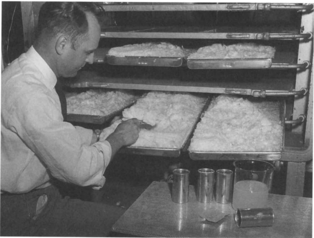
Figure 10.17. Batch-type vacuum shelf drier. Source: Ponting et al., Food Dehydration, 2nd ed., Vol. 2, W.B. Van Ardel, M.J. Copley, and A.I. Morgan, Jr. (Editors). AVI Publishing Co., Westport, CT, 1973.
